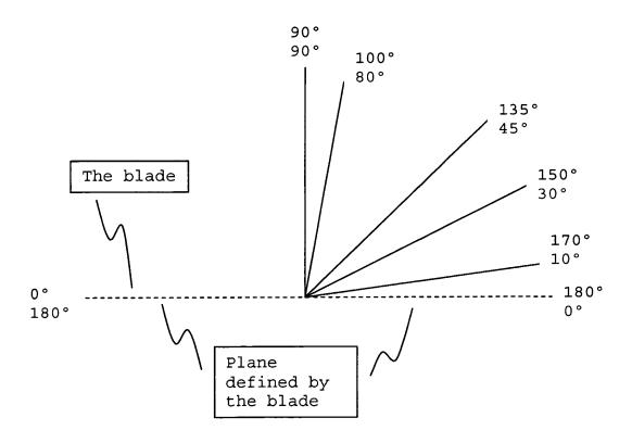
It is submitted that depending on where the zero point is established for the plane defined by the blade, various angles can represent the same orientation of the angle between the blade portion and the handle portion of the utility knife, as defined by the present claims. For the sake of clarity, claim 4 has been amended to recite that the angulation ranges from about 100 degrees to about 170 degrees. Claim 5 has been
